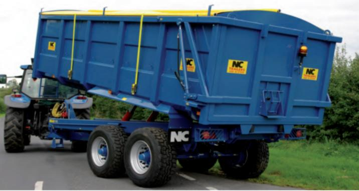
The 10 and 12 Ton models are fitted with a 40kph axle while 13 -25 Ton models are fitted with high speed axles with 420x180 brake drums as standard. Standard wheel is the 385/65x22.5 super single. All trailers are fitted with an automatic top hinged tail door, complete with grain chute and manual securing bar. **See optional extras**
