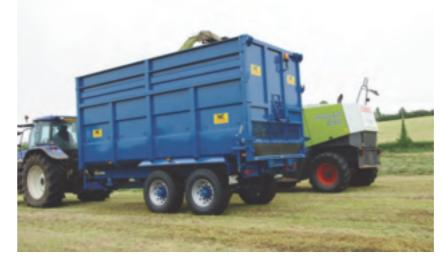
NC Engineering offer a selection of Silage/Grain trailers ranging from 10-25 Ton capacity. The monocoque body comes with a 100mm front to rear taper and tips to an angle of 50 degrees to ensure easy emptying.
